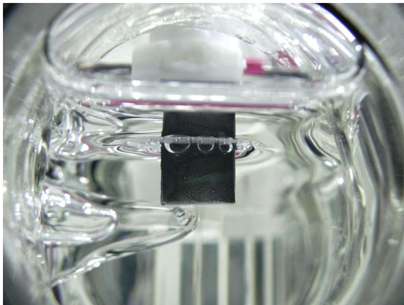
Figure S10. Enlarged digital photograph showing oxygen evolution from the truncated \text{In}_2\text{O}_3 octahedral electrodes taken at 60 min (amperometric I - t curves).
