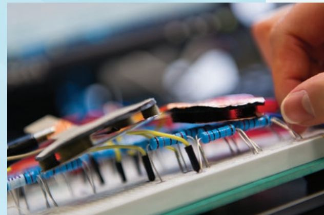
The energy harvesting device charges mobile electronics by converting mechanical into electrical energy. 城大研製的能量收集裝置將動能轉為電能，為手提電子產品充電。
