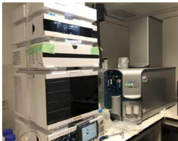
Agilent 1290 Infinity UPLC equipped with SCIEX X500R QTOF MSMS
