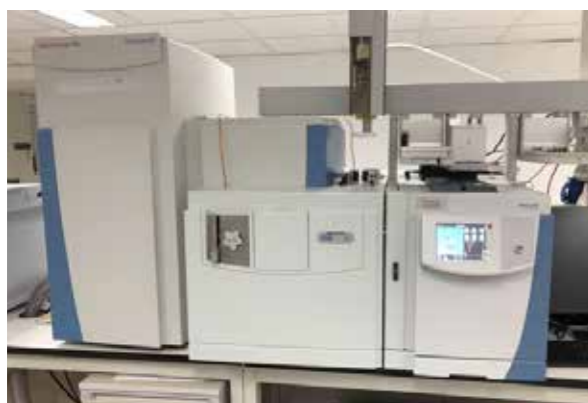
Thermo Fisher Q Exactive GC Hybrid Quadrupole-Orbitrap Mass Spectrometer
